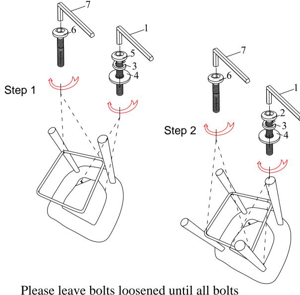
Please leave bolts loosened until all bolts are placed before tightening completely
