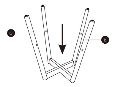
Attach the Footrest (D) to the assembled stool base in Step 1. Loosely attach the first Long Bolt (F) and move onto attach the diagonal Long Bolt (F), one by one. After all bolts are attached, use Allen Wrench (K) to fully tighten.
