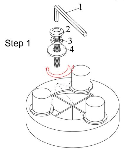
Please leave bolts loosened until all bolts are placed before tightening completely
